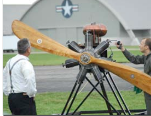
Tom Kozura gets the 1909 50-hp Gnome engine ready for a demonstration run.
