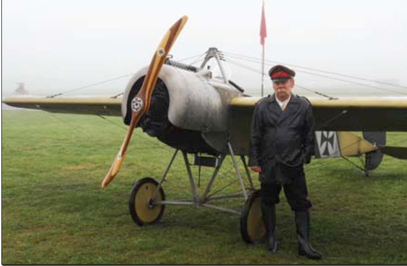
Eric Williams with his modified Airdrome Aeroplanes Fokker E-III. Power is supplied by a Geo engine with cog-belt reduction. Note the foggy conditions. The windsock is limp, and you can't see the museum's hangars in the background.
